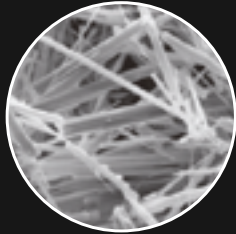
Crystalline structure of calcium sulfate \alpha -hemihydrate
